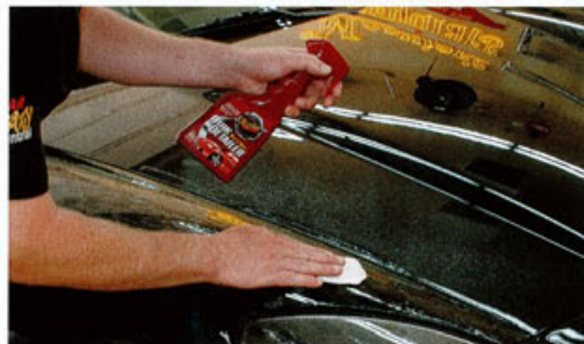
Tree sap, hard-water deposits, and other above-the-surface contaminants can be removed using a clay bar. Make sure to lubricate the surface before rubbing it with the bar. Though it's typically used as a between-washes cleaner, Meguiar's Quik Detailer offers enough lubricity to be used with the clay.
