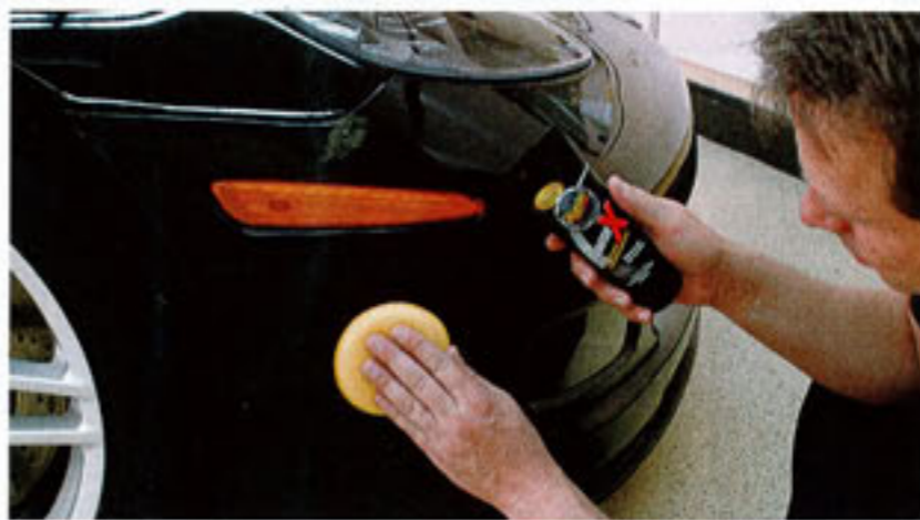
Below-the-surface imperfections, such as swirl marks, can be eliminated using a cleaner/swirl-remover like Meguiar's ScratchX. Unlike some conventional compounds, ScratchX is safe to use on any automotive paint and clearcoat, thanks to its "diminishing abrasive technology." Developed by Meguiar's, these abrasive particles get smaller and smaller as you work them into the paint.
