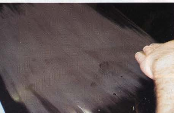
(left) Which grit sanding paper you start with depends upon the severity of the damage. Our panel has lots of scratches, but nothing very deep, so we started with 2,000 Unigrít Finishing Paper from Meguiar's, backed by their sanding pad. The unique feature of the Unigrít paper is that the particle size is uniform, as is the distribution. This guarantees that every pass removes the same amount of material. (right) Using a clean spray bottle with water and high-lubricity car-wash soap, spray the work area and begin to sand using a light, straight-line sanding technique and check your progress frequently.
