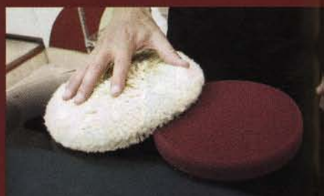
Now it's on to Step 2- Removing sanding marks. In this step, we'll be using a rotary machine buffer with either a wool or foam cutting pad to apply the compound. We opted to use the Cut 'N Shine Wool Pad since it's a little more aggressive in removing imperfections than the burgundy colored Soft Buff cutting pad.
