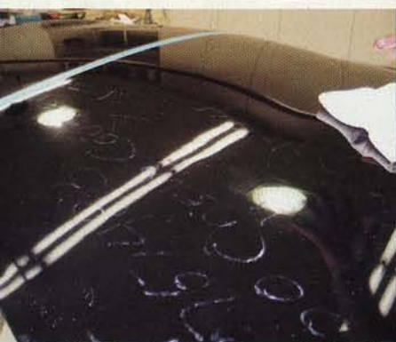
With the area washed clean and dried, the inspection process can begin. Adequate lighting is important so that every imperfection can be viewed. Notice how the reflection of the halogen light looks blurry? That's caused by orange peel. The process we will use to remove the scratches and swirls will also knock some of that down.
