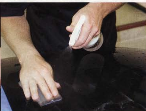
(left) Which grit sanding paper you start with depends upon the severity of the damage. Our panel has lots of scratches, but nothing very deep, so we started with 2,000 Unigrít Finishing Paper from Meguiar's, backed by their sanding pad. The unique feature of the Unigrít paper is that the particle size is uniform, as is the distribution. This guarantees that every pass removes the same amount of material. (right) Using a clean spray bottle with water and high-lubricity car-wash soap, spray the work area and begin to sand using a light, straight-line sanding technique and check your progress frequently.
