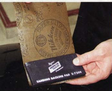
(left) Which grit sanding paper you start with depends upon the severity of the damage. Our panel has lots of scratches, but nothing very deep, so we started with 2,000 Unigrít Finishing Paper from Meguiar's, backed by their sanding pad. The unique feature of the Unigrít paper is that the particle size is uniform, as is the distribution. This guarantees that every pass removes the same amount of material. (right) Using a clean spray bottle with water and high-lubricity car-wash soap, spray the work area and begin to sand using a light, straight-line sanding technique and check your progress frequently.
