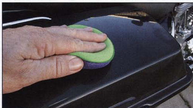
8 Tech Wax paste works on painted metal parts as well as fiberglass saddlebags and fairings.
